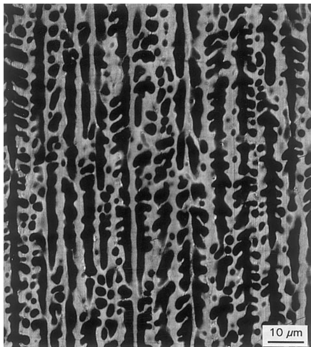
Figure 13 Backscattered scanning electron image (longitudinal section) of Al-7%Y alloy wire showing dendrite structure. Casting speed was 0.2 \text{ m min}^{-1} .
